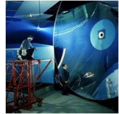
Photo: Now that's what I call a mirror! A solar mirror used to gather and focus energy from the Sun. Picture by courtesy of NASA Glenn Research Center (NASA-GRC).
